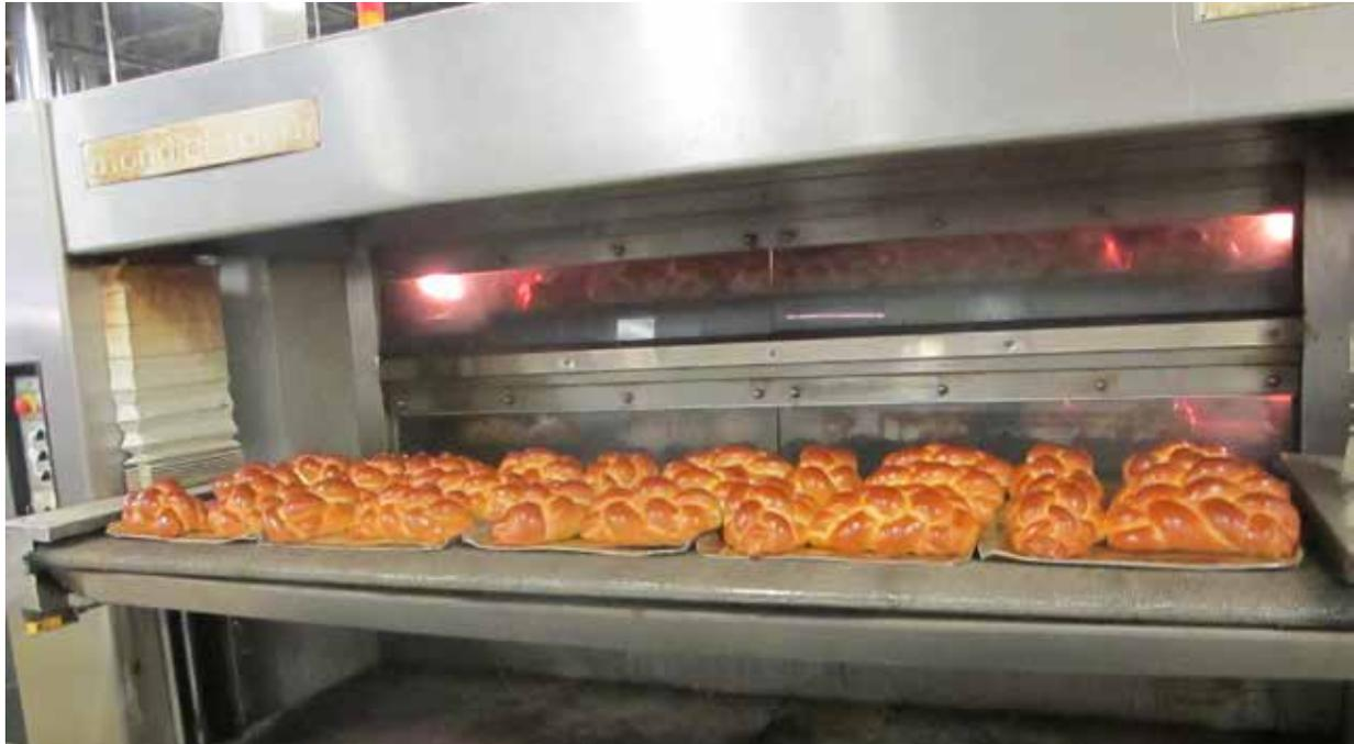
Freshly baked loaves of challah bread leave the three-deck tunnel oven, then are racked and cooled before packaging.
